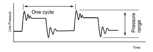
Figure 1 : Pressure Cycle
